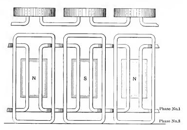
FIG. 64. Diagram of two-phase winding using several forms of coil.
